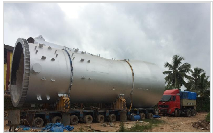
Stack Module (5.6 \phi x 4.5 \phi x 15.5 Mtrs)
